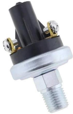
ZTUOAUMA 10PSI±2PSI Oil Pressure Switch 0C3025 1/4- 18 NPT Normally Close
