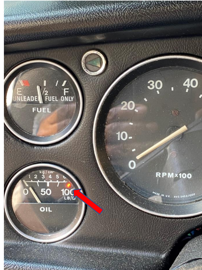
Oil Pressure Light On, Ignition On
